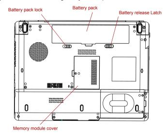
Figure 2-5 The underside of the computer
